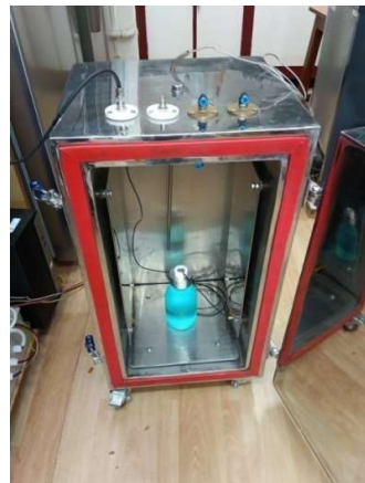
Fig. 2 The temperature controlled system (TCS) and the detector (SLD)
