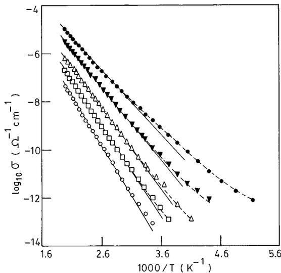
FIG. 1. Temperature dependence of the dc conductivity for bismuth cuprate glasses: ○, 27.15 mol % CuO; □, 35.35 mol % CuO; △, 45.70 mol % CuO; ▼, 55.62 mol % CuO; ●, 67.60 mol % CuO. The solid lines are the best fits of the data above 300 K to Eq. (1). The dashed curves are drawn through the data to guide the eye.
