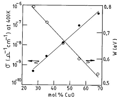
FIG. 3. Composition dependence of the conductivity at 400 K (●) and high temperature activation energy (○) for the bismuth cuprate glasses.
