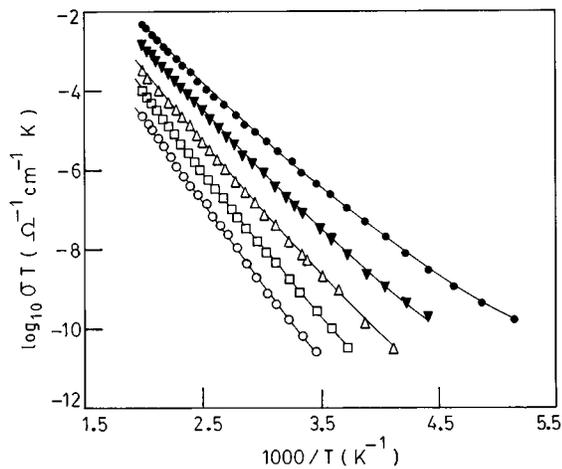
FIG. 5. Plots of  $\log_{10}(\sigma T)$  vs  $10^3/T$  for the same bismuth cuprate glass compositions as in Fig. 1. The solid curves are the best fits to Eq. (11).
