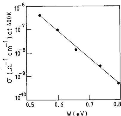
FIG. 4. Plots of  $\log_{10}\sigma$  vs  $W$  at 400 K for different compositions of the bismuth cuprate glasses. The solid straight line is the least square fit to the data yielding a temperature of 440 K.
