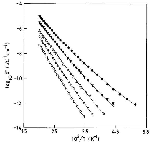
FIG. 6. The fits of the measured dc conductivity to the prediction of Emin's model [Eqs. (12) and (13)]. The solid curves represent the best fits for the same sample compositions as in Fig. 1.
