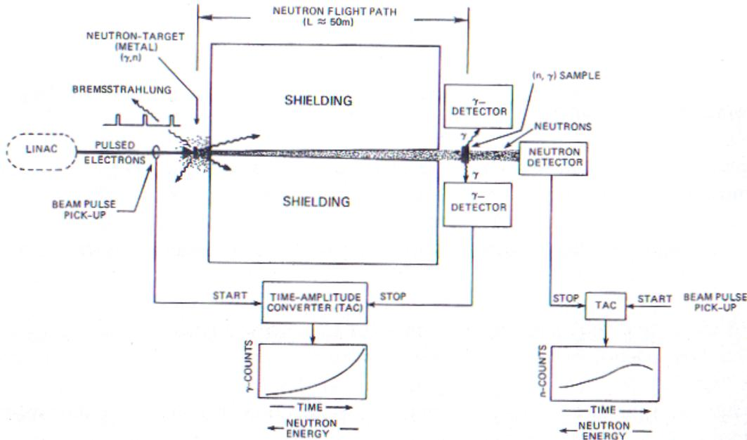
Schematic layout of TOF measurement;
