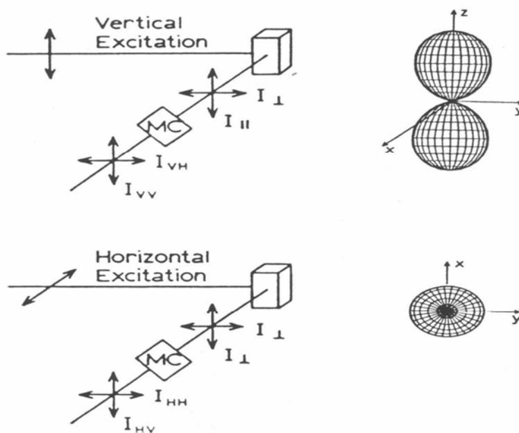
**Figure 3** Schematic diagram for L-format measurements of fluorescence anisotropy. (MC is the monochromator). The shapes at the right are the excited state distributions.
