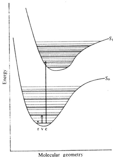
**Figure 1** *Energy levels of a small molecule. Selected rotational sublevels of the vibrational levels of each of two electronic states are shown. Transitions corresponding to electronic (e), vibrational (v) and rotational (r) spectra are indicated.*
