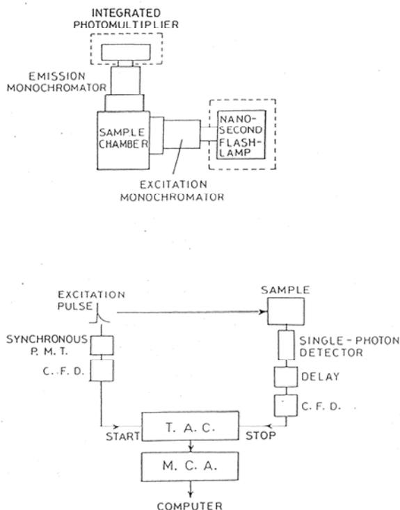
**Figure 4** *Block diagram of the TCSPC set-up*
