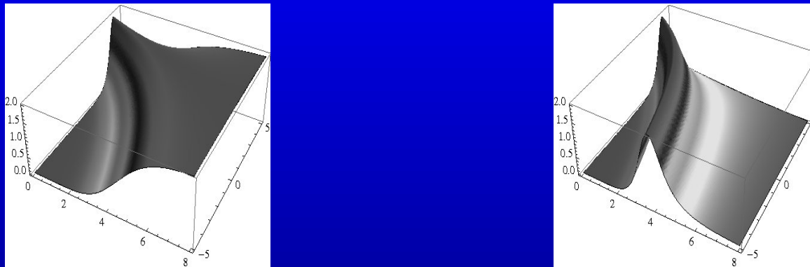
Figure 4: a) Broadening of optical soliton |E(z, t)| moving along the fiber. b) Efficient control of the soliton broadening by coupling to double SIT system, showing restoration of the soliton width and constant change in the soliton velocity.
