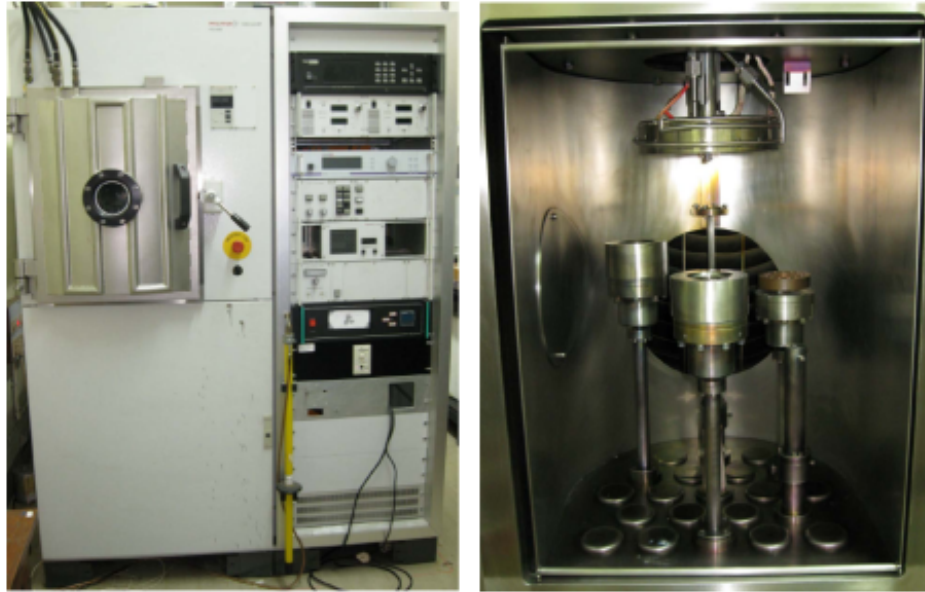
Figure 12: Left: Magnetron sputtering instrument (PLS 500). Right: Inside view of the deposition chamber
