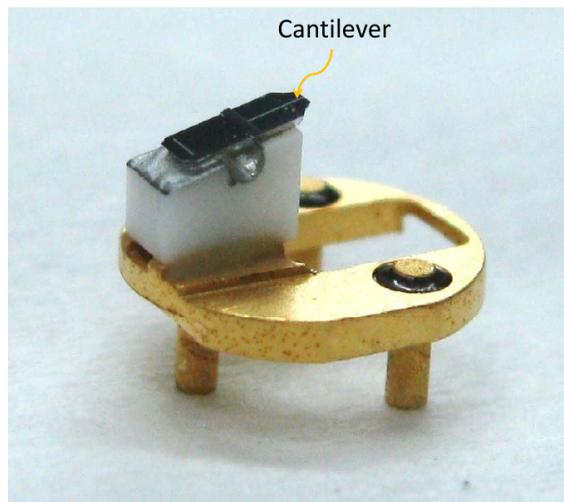
Figure 3.14: Picture of AFM tip stage of UHV-SPM
