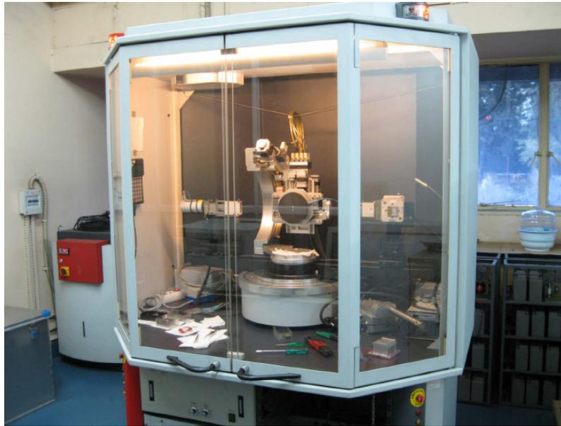
Figure 3.7: Picture of VXR instrument used in x-ray reflectivity measurements.
