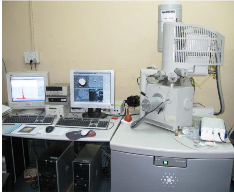
Figure 3.19: Picture of a SEM instrument.
