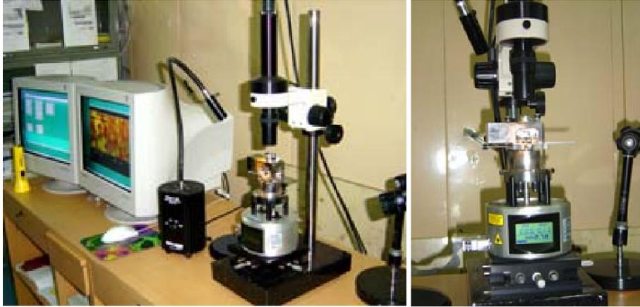
Figure 3.16: Picture of ambient AFM instrument (Nanoscope-IV, Veeco).
