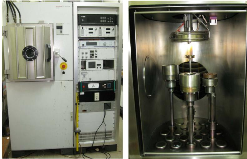
Figure 3.2: Picture of Magnetron sputtering instrument (PLS 500) shown in left side. Inside view of the deposition chamber shown in right side.
